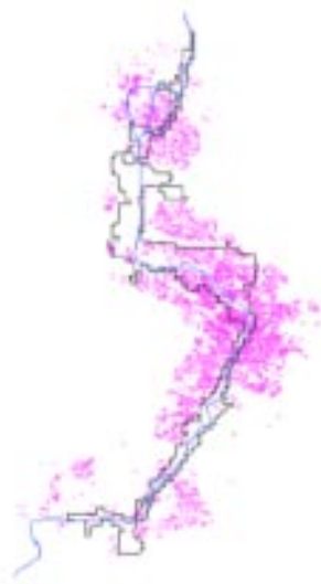
Figure 7. The affected buildings (within the polygon) with a 100 year flood event.
