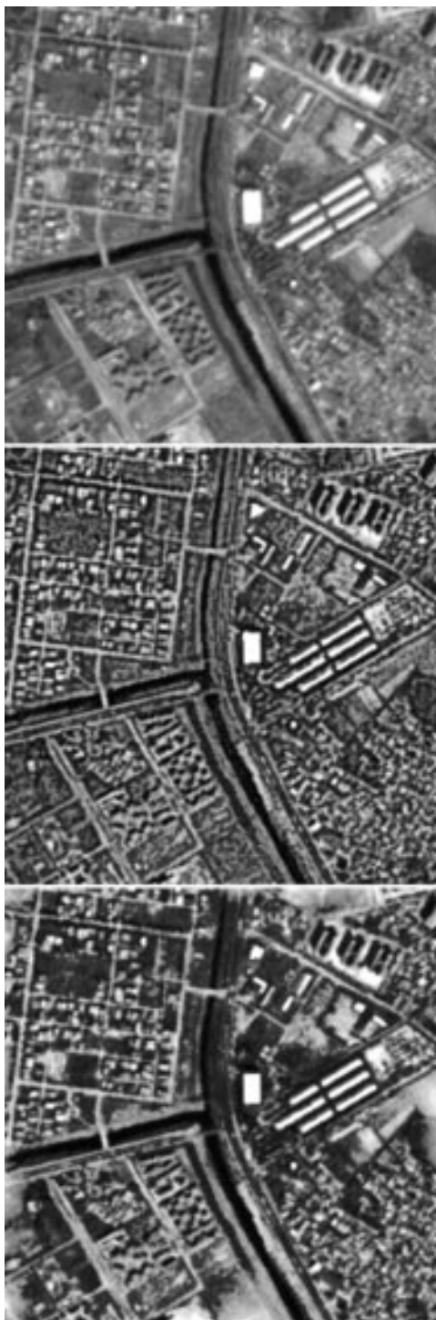
Figure 6: Top – Linear stretched remote sensing image, Middle – Local contrast enhancement by Beghdadi's method, Bottom – Local contrast enhancement by proposed method with \sigma = 0.4 for DoG.
