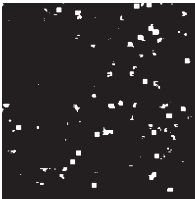
Fig 3 Edges detected by variance filter
