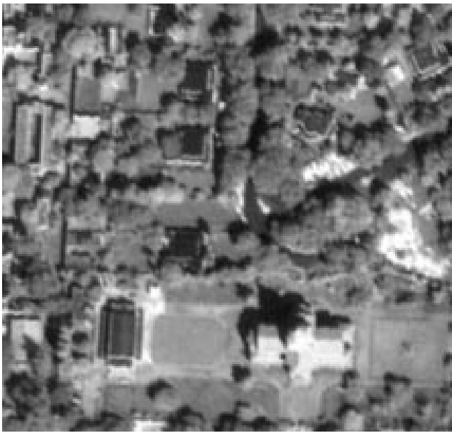
Figure-11: 60° rotated 2 m image, registered with respect to original (GSD=1 m)
